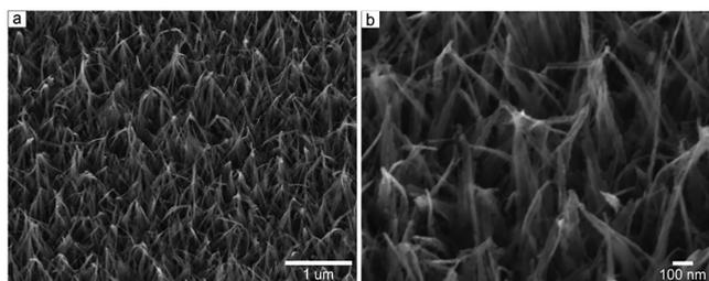
**Figure 1.** SEM images of hydrothermally synthesized nanostructured TiO<sub>2</sub> surface at various magnifications.
