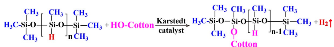
Scheme 1. Reaction of poly(methylhydrogen)siloxane (PMHS) with cotton fabric.
