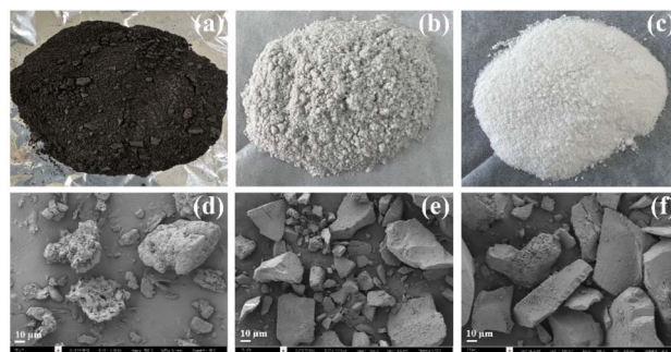
Fig. 1 Photographs of powder and SEM images of as-received SCBA (a and d), SiO 2 -P (b and e), and SiO 2 -PS (c and f).
