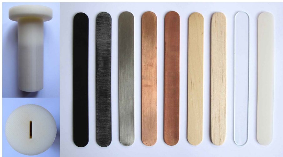
Figure 1. The nine stimuli used in the study, with one of the weighted ABS handles used to hold the stimuli during the experiment. From left to right: polystyrene (PS), rough polystyrene (R PS), stainless steel, copper, rough copper, birch, balsa, glass and silicone. doi:10.1371/journal.pone.0105035.g001
