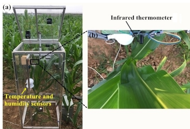
Figure 2. Photos of leaf temperature, air humidity, and temperature sensors in the chamber: (a) location of the sensors within the chamber and (b) location of the leaf temperature sensor.
