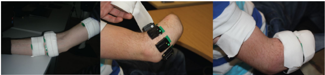
Fig. 4 Sensor placement on able-bodied (left) and amputee subjects (centre, right) [20]. Eight EMG-IM sensors are equally spaced around the participants' forearm (3 cm below the elbow). Two are place on
