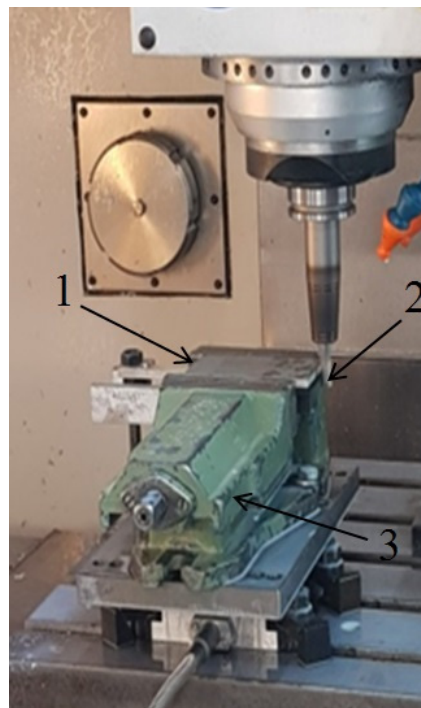
Figure 3. Milling of a sandwich structure: 1. sample, 2. tool, 3. machine vice.
