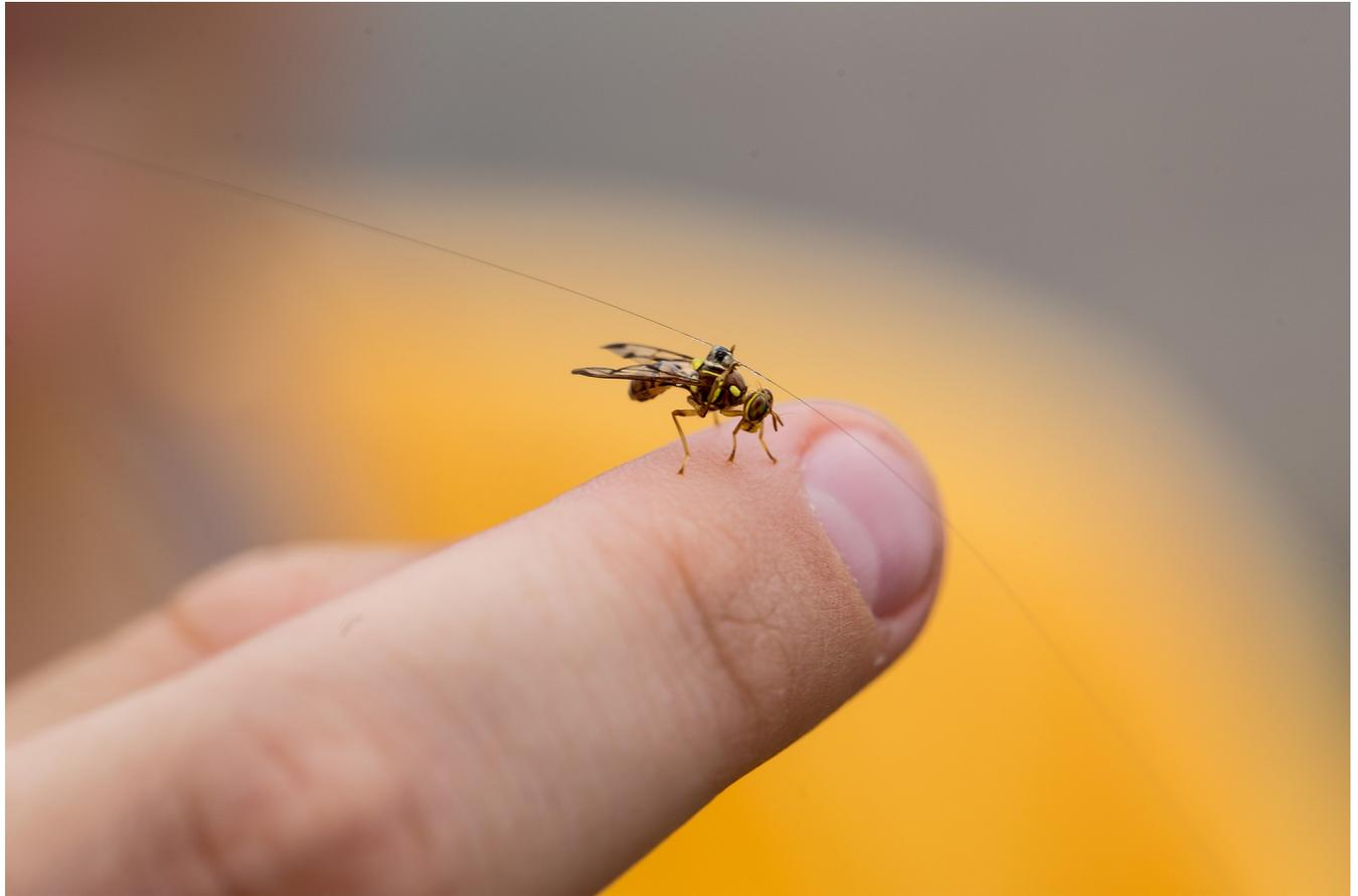
**Fig 1. A wild male melon fly, *Zeugodacus cucurbitae*, with a harmonic radar tag attached.** The tag shown weighed approximately 0.8 mg and was fabricated from a diode and superelastic nitinol wire.
