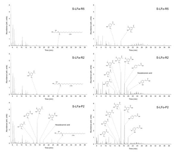
**Figure 6.** GC/MS total ion chromatograms of delivered fractions from aqueous and organic processes using S-LFa/o-0. Selected component identification by MS library matching is reported for each fraction.
