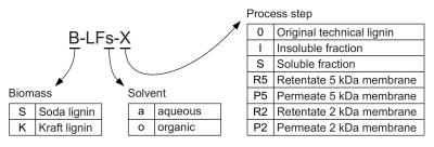
Figure 2. Labelling scheme for lignin fractions.
