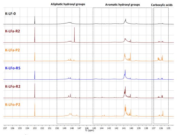
**Figure 9.** <sup>31</sup>P-NMR spectra of lignin fractions recovered from the aqueous and the organic process applied on K-LF-0.
