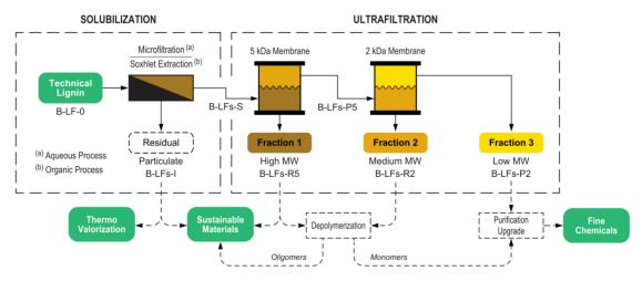
**Figure 1.** Overview of the overall fractionation process. Possible applications of obtained fractions and related downstream processes are indicated in the bottom line (dashed arrows).
