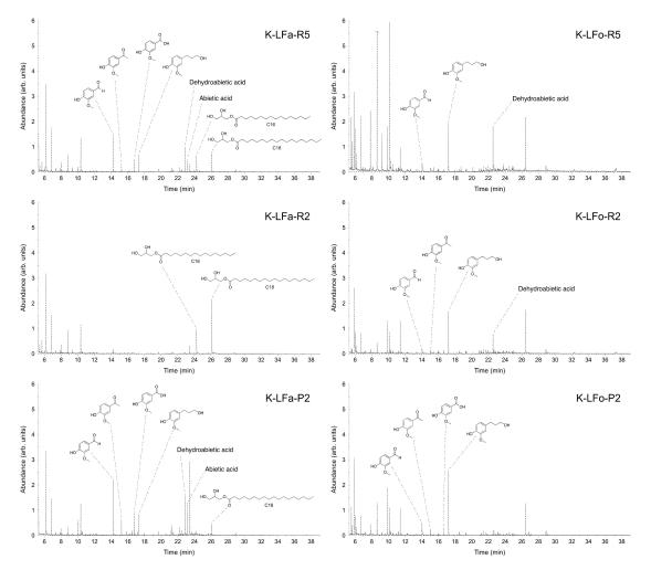
**Figure 7.** GC/MS total ion chromatograms of delivered fractions from aqueous and organic processes using K-LFa/o-0. Selected component identification by MS library matching is reported for each fraction.
