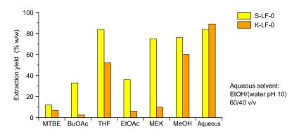
**Figure 3.** Extraction yields as the percent (w/w) of solubilized fraction vs. total fraction for S-LF-0 (yellow) and K-LF-0 (orange) for different organic solvents and for the (basic) aqueous system.
