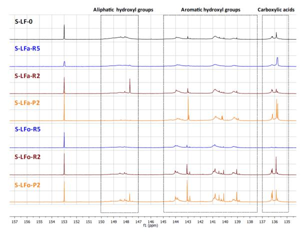
**Figure 8.** <sup>31</sup>P-NMR spectra of lignin fractions recovered from the aqueous and the organic process applied on S-LF-0.
