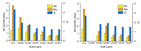
**Figure 4.** Comparison of the results of the aqueous and organic processes for S-LF-0 and K-LF-0 fractionation as Mn, Mw, and *D* by GPC analysis of resulting delivered fractions.
