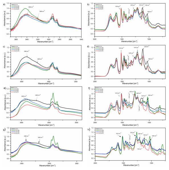
**Figure 10.** FT-IR spectra of soda (**a**,**b**,**c**,**d**) and kraft (**e**,**f**,**g**,**h**) lignin fractions recovered from the aqueous process (**a**,**b**,**e**,**f**) and the organic process (**c**,**d**,**g**,**h**). Different regions of the infrared spectrum are reported for clarity.
