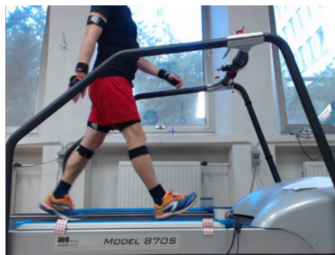
Figure 1. Acquisition of the subject wearing the Xsens (MVN awinda, Netherlands) full mocap system while walking between the optical bars, Optogait™ (Microgait, Italy) on the treadmill (Medisoft, Model 870S, Belgium) at an imposed speed of 5 km/h.
