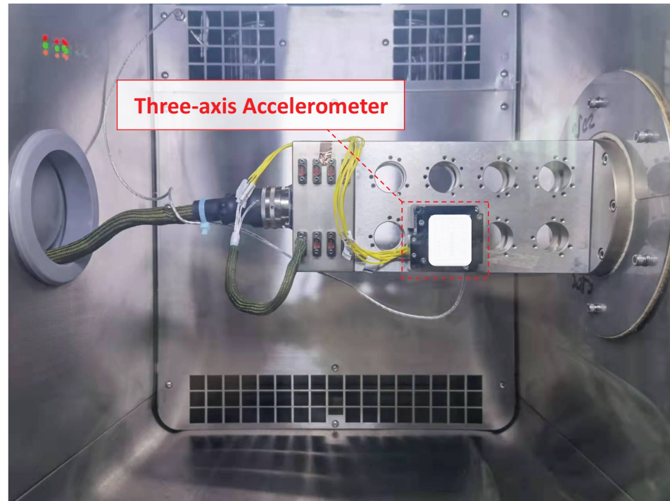
Figure 3. Experimental platform of accelerometer for temperature compensation.
