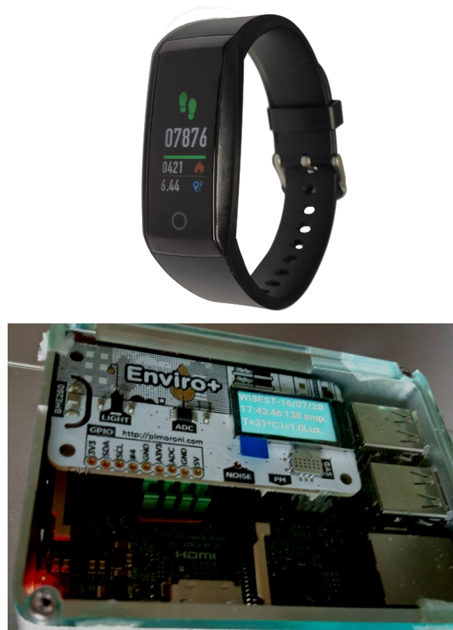
Figure 1. Some devices implemented in the case study 1. Smartbands to collect stress levels on top subfigure and Single Board Computers with appropriate plugin sensors on bottom subfigure.
