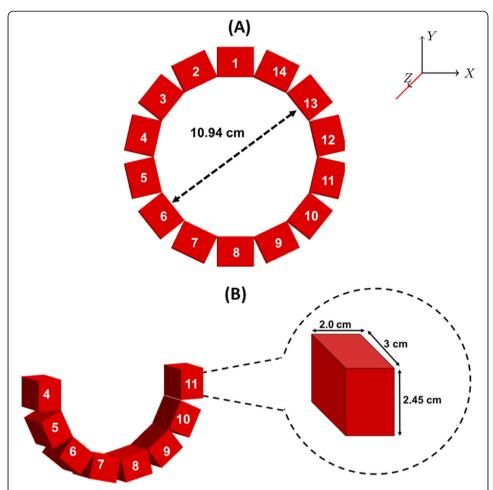
**Fig. 2** Schematic detailing layout of the wristPET1 (**a**) system. wristPET1 consists of 14 detectors in a closed ring design, whereas a second system (wristPET2 (**b**)) was projected to employ an open-ring design with a subset of detectors (numbers 4-11) only. All other properties of the detectors between wristPET1 and wristPET2 are identical
