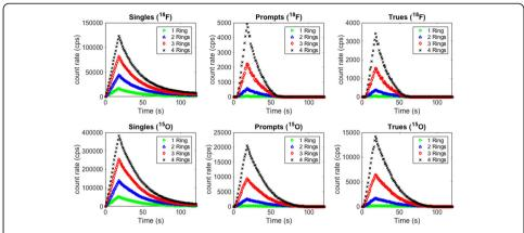
**Fig. 7** Total singles, prompt, and true event rates for wristPET2 system simulated for an increasing number of detection rings (1, 2, 3, and 4) for <sup>18</sup>F simulation (top row) and <sup>15</sup>O simulation (bottom row). All variables were constant except the number of detection rings
