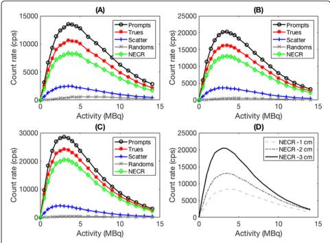
**Fig. 5** Count rate performance of the wristPET2 (8 detector system) using a point source at different Y-positions inside an 8-cm-diameter water phantom at  ${\bf a}$  Y=-1 cm below center,  ${\bf b}$  Y=-2 cm below the center, and  ${\bf c}$  Y=-3 cm below the center of the scanner  ${\bf d}$  comparison of NECR at Y=-1 cm, Y=-2 cm, and Y=-3 cm where NECRmax is 8360 cps, 13041 cps, and 20,476 cps at an activity of 3.5 MBq
