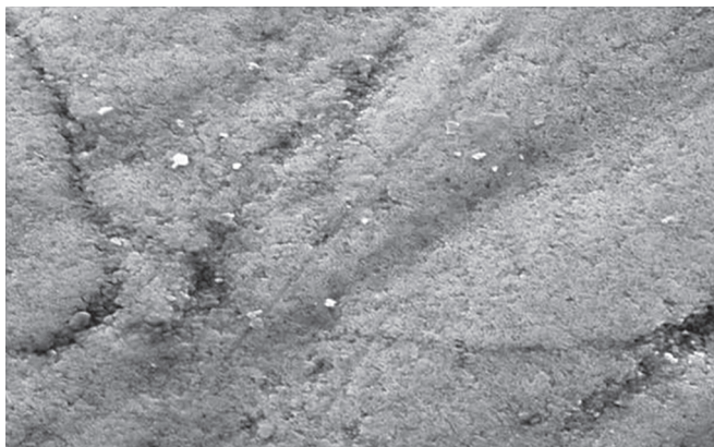
Fig. 3: Structural analysis of remineralized enamel sample treated with CPP-ACP paste by SEM
