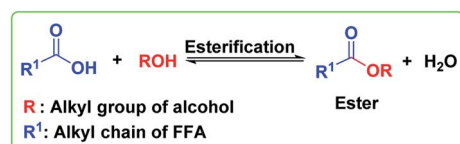
Scheme 2 Acid-catalyzed esterification of FFA content of vegetable oil to biodiesel.
