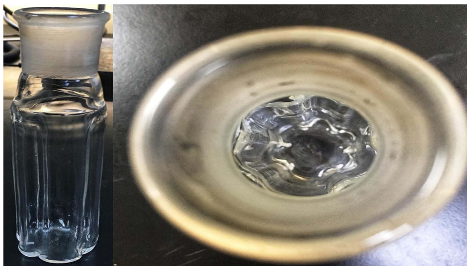
Figure 1 The six-baffled homemade glass vessel simulating Mozafari's glass bottle.
