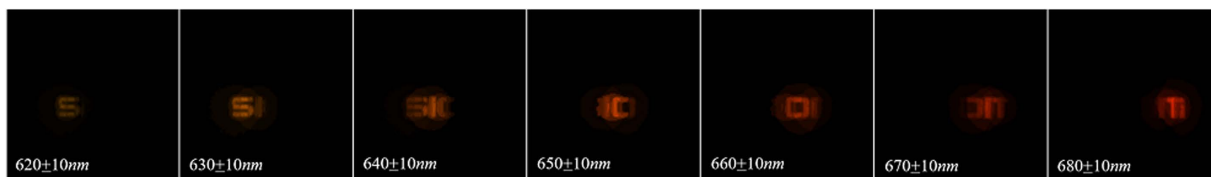
Figure 4. The original spectral images of ‘SIOM’ obtained by CCD1 detector placed on the first image plane ‘b’ with corresponding narrowband filter in front of it, showing all the channels from 620 ~ 680 nm.
