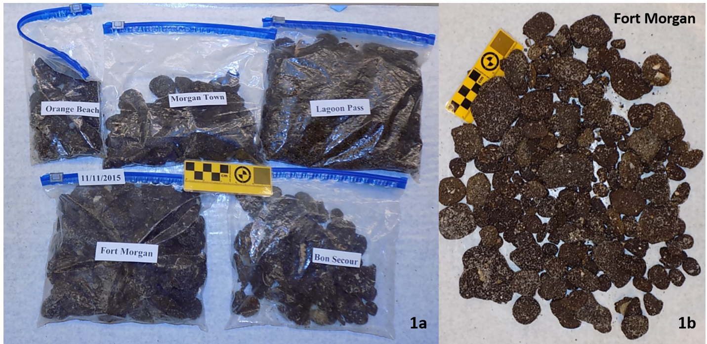
Fig 1. Oil spill residues collected from five different Alabama beaches on November 11th 2015 in the left side picture and residues collected from Fort Morgan (218 samples of total weight 836 grams; sampling distance ~1 km, and sampling time ~1 hour) in the right side picture.
