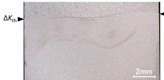
**Figure 6.** The macroscopic fracture surface of the additional test sample.
