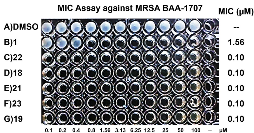
Figure 3. MIC assay results of potent new HPs (MIC = 0.10 \mu\text{M} ) against MRSA BAA-1707.
