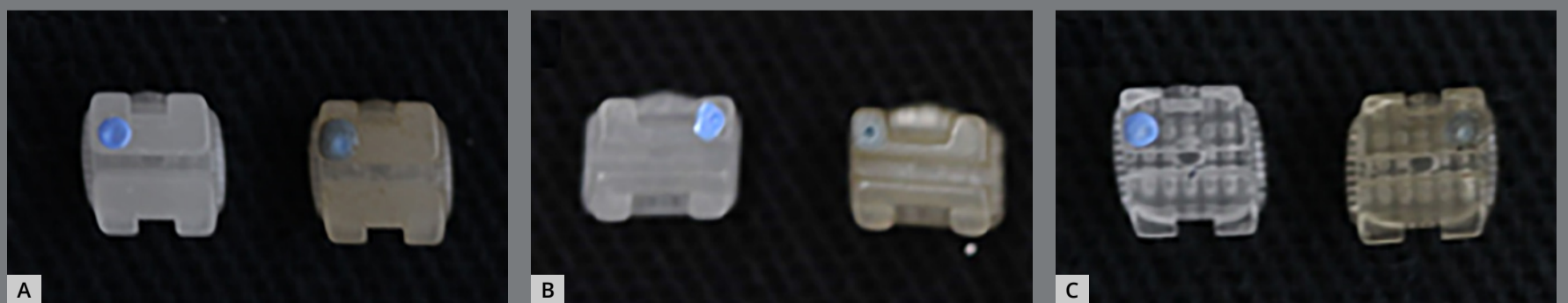
Figure 6: Photograph of aesthetic brackets: ceramic (A), composite (B) and polysafira (C) before and after exposure to smoke.
