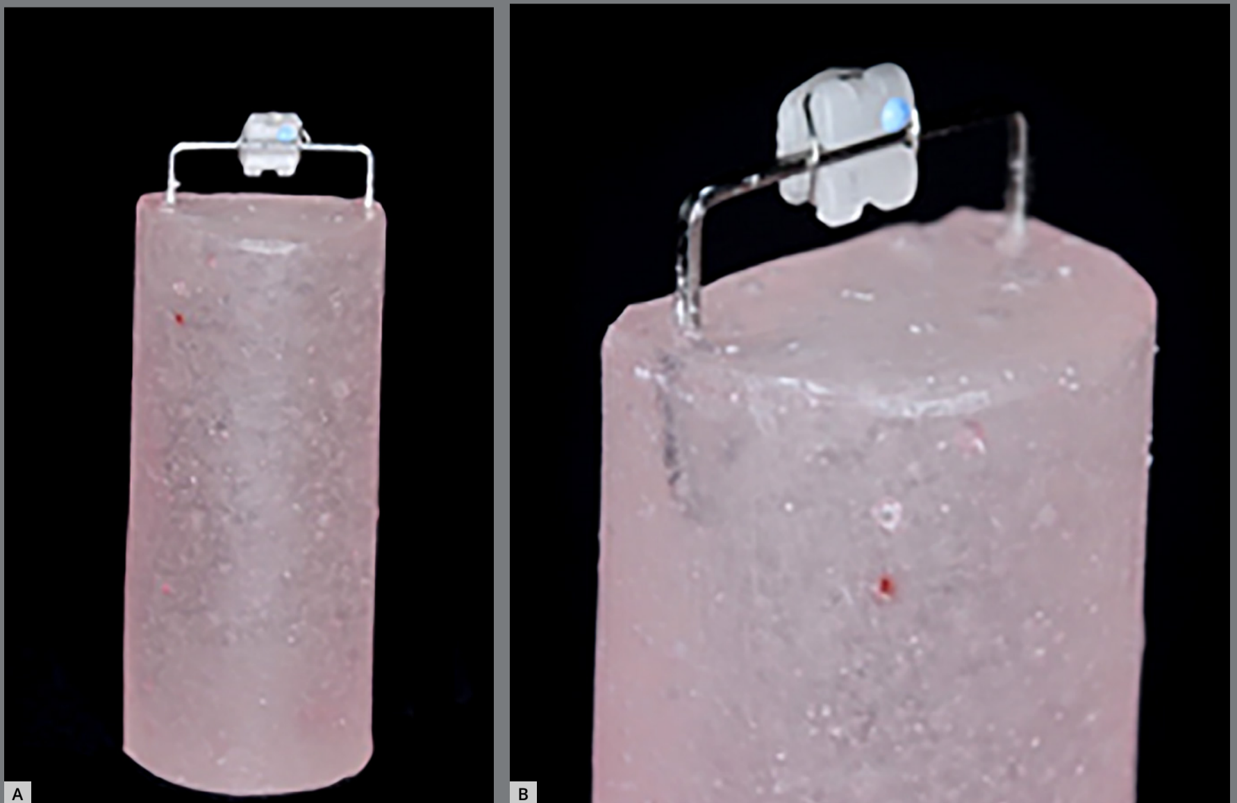
Figure 1: Photograph of specimens produced with steel wire (A); bracket tied to the specimen wire (B).
