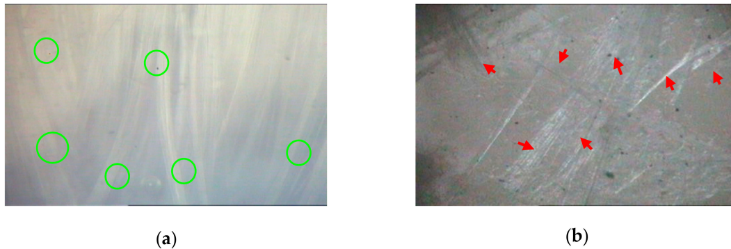
Figure 2. The optical morphologies of chrysotile fiber: (a) in bundle (green circles) ( \times 200 ); (b) dispersed state in ethanol (red arrows) after grinding for 30 min ( \times 200 ).
