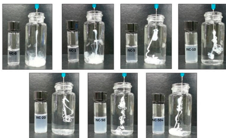
Figure 6. Appearances of the liquefied 15% ( w/v ) PNIPAAm-CNC hydrogel samples with different CNC loadings before injection (small glass vials) and their appearance changes during their injection into 37 °C water bath (large glass vials).
