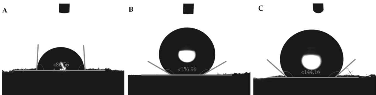
Figure 2. Goniometrical analysis of wettability performed for (A) PUF, (B) MTMS aerogel and (C) PP fibers.
