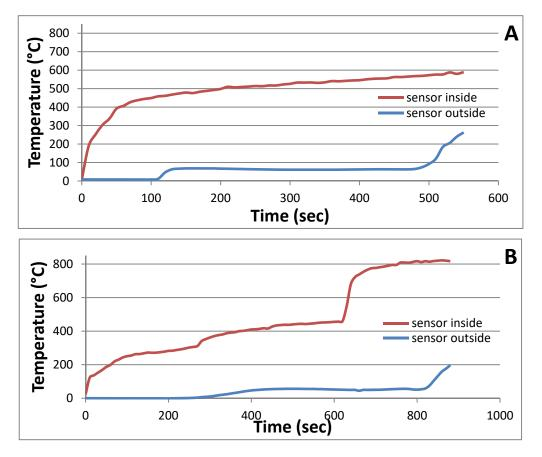
Figure 8. Burning characteristics of produced panels: (A) Rapid temperature increase; (B) gradual temperature increase.
