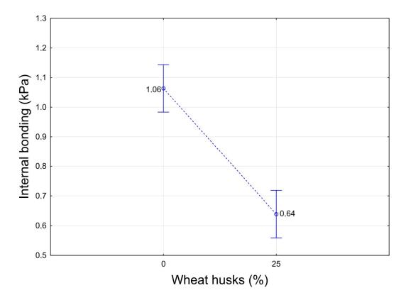
**Figure 7.** Influence of the proportion of the husk in the insulation board on internal bonding of composite materials.
