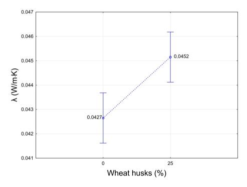
**Figure 5.** Influence of the proportion of the husk in the insulation board on the thermal conductivity coefficient.
