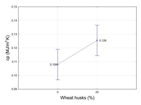
Figure 6. Influence of the proportion of the husk in the insulation board on volumetric heat capacity (cp).
