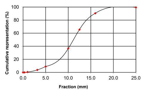
Figure 3. Fraction of crushed PUR foam.
