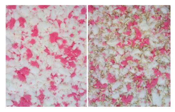
**Figure 1.** Surface view of the thermal insulation layer, board without husks on the **left**, board with addition of husks on the **right**.
