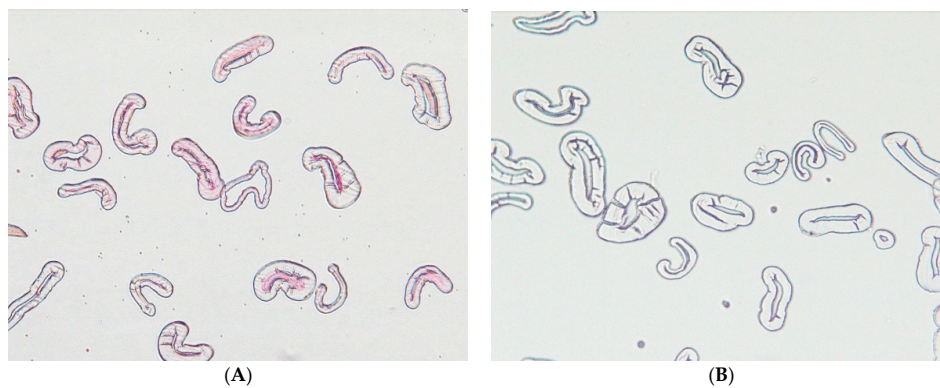
Figure 1. Microscope images of cross-sectioned cotton fibers after staining with Ruthenium Red are (A) hydroentangled (HE) brown nonwoven greige cotton and (B) scoured and bleached cotton fiber. Note: The brown cotton fiber was distinctively stained.
