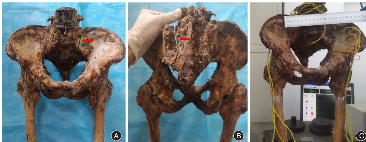
Fig. 4 Posterior pelvic ring fracture models and the testing machine used in this study. (A) Six embalmed adult male cadaveric pelvises (viewed from the front) were cut from the midpoint of the sacroiliac joint and sacral foramen to create posterior pelvic ring fracture models. The fracture line is indicated by the red arrow. (B) The pelvic specimens viewed from behind. The fracture line is indicated by the red arrow. (C) The pelvic specimens were placed in the biomechanical testing machine
