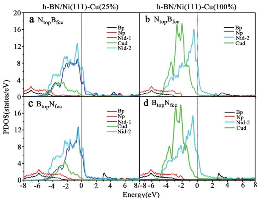
Fig. 6 Projected densities of states (PDOS) of B, N, Ni and Cu atoms for monolayer h-BN on (a and c) Ni(111)-Cu(25%) and (b and d) Ni(111)-Cu(100%) surfaces for the (a and b)  $N_{\text{top}}B_{\text{fcc}}$  and (c and d)  $B_{\text{top}}N_{\text{fcc}}$  stacking configurations.
