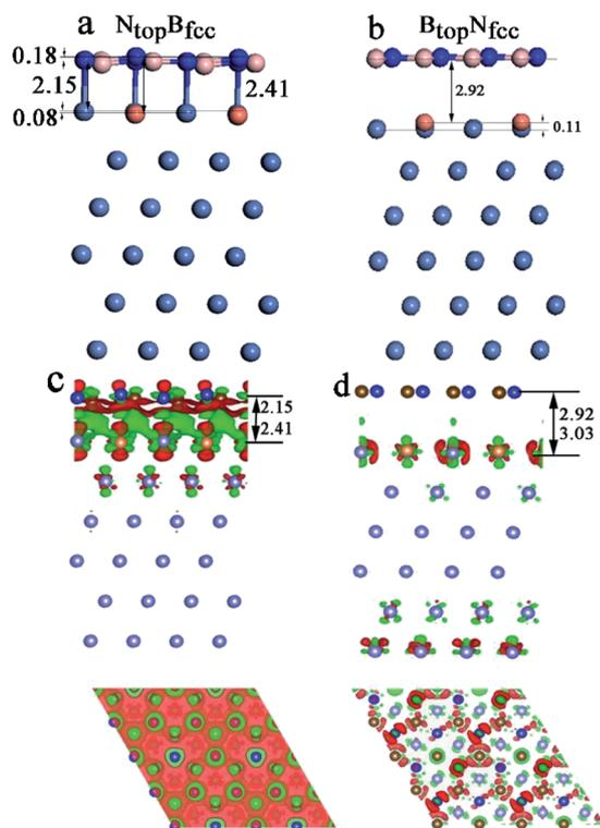
Fig. 4 Optimized geometric structures (a and b) and charge density difference plots (c and d) of monolayer h-BN adsorbed on Ni(111)–Cu(25%). Pink, blue, gray, orange and purple represent B, N, C, Cu and Ni atoms, respectively. The positive and negative charge are shown in red and green on the charge density isosurfaces, respectively.
