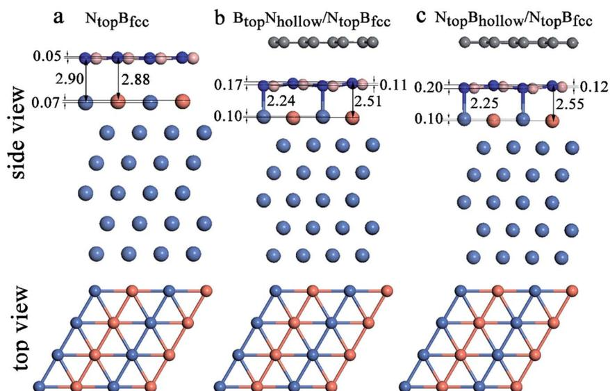
Fig. 8 Optimized stable adsorption configurations of (a) the h-BN/Ni(111)-Cu(50%) with  $N_{\text{top}B_{\text{fcc}}}$  stacking, (b) 1L-Gr/h-BN/Ni(111)-Cu(50%) with  $B_{\text{top}N_{\text{hollow}}/N_{\text{top}B_{\text{fcc}}}$  stacking and (c) 1L-Gr/h-BN/Ni(111)-Cu(50%) with  $N_{\text{top}B_{\text{hollow}}/N_{\text{top}B_{\text{fcc}}}$  stacking.
