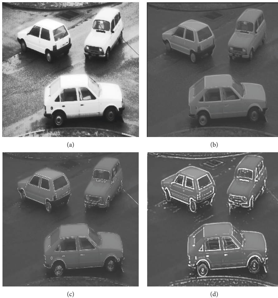
FIGURE 9: Enhancement effects of various algorithms. (a) Region growing-based image enhancement. (b) Operator-based image enhancement. (c) PST-based image enhancement. (d) Fractional-order PST-based image enhancement.
