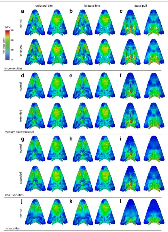
Fig. 2 Von Mises stress contour plots for different tested cranial configurations: **a–c** original model, **d–f** medium-sized interpterygoid vacuities, **g–i** small interpterygoid vacuities, **j–l** closed palatal region.
