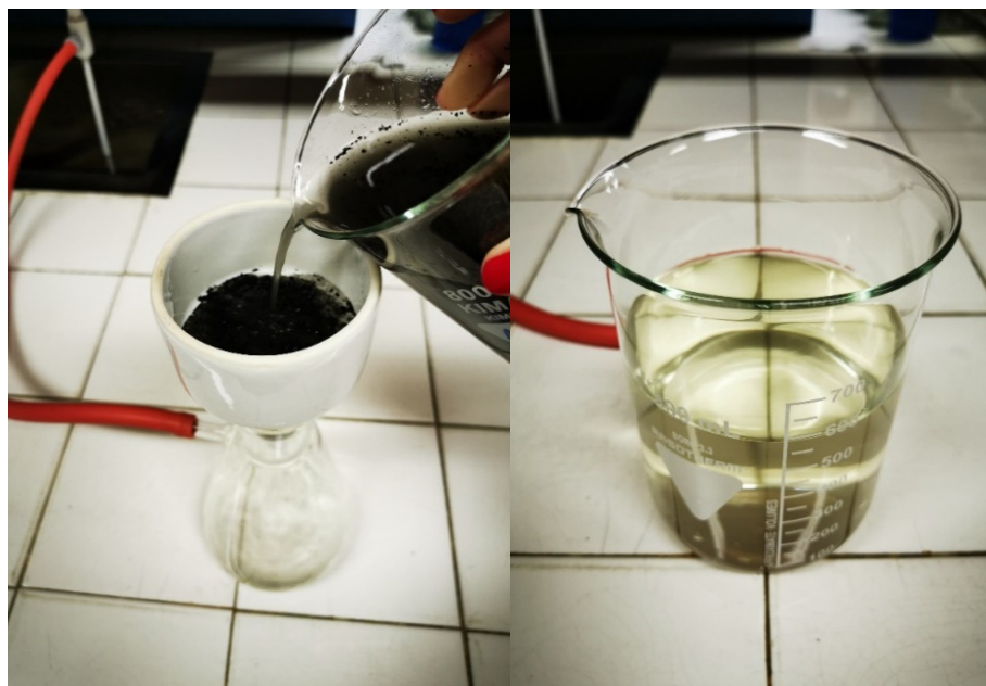
Figure 2. Preparation of wood ash extract: vacuum filtering the solution (left) and wood ash extract (right).
