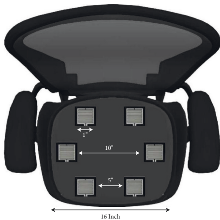
FIGURE 3: Arrangement 01, six sensors arrangement on a chair.
