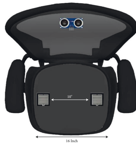
FIGURE 4: Arrangement 02: two FSR and one ultrasonic sensor.
