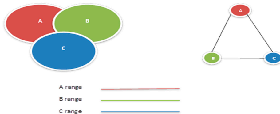
Figure 2. Wireless network and the corresponding graph model.
