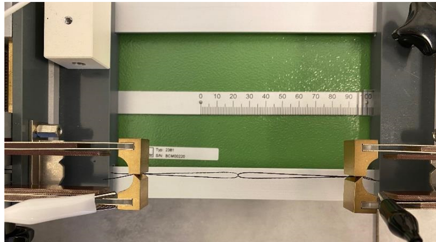
Figure 4. Image of the real measurement set-up of the interlooped sensory yarns.
