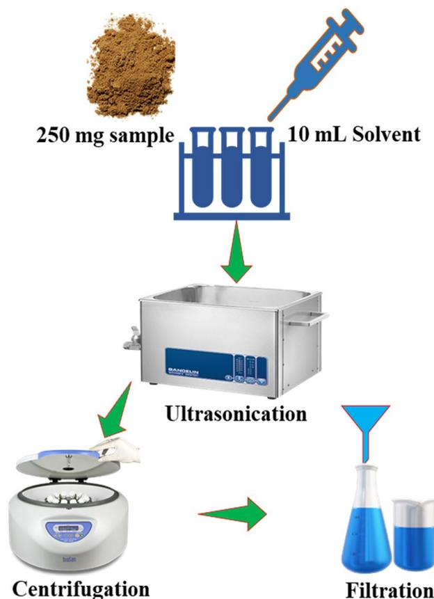
**Figure 2.** A schematic diagram for extraction process.
