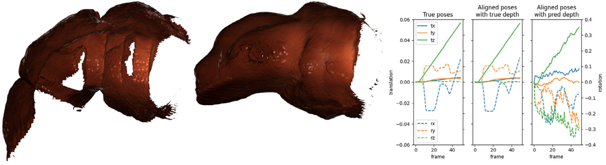
FIGURE 7 3D shape reconstruction results. The reconstructed shape from 50 frames of the true depth map (left) and the predicted depth map (middle), and the true poses and the estimated poses are compared (right). The rotation parameters are in the axis-angle representation. Back faces are culled off for visualizing meshes.
