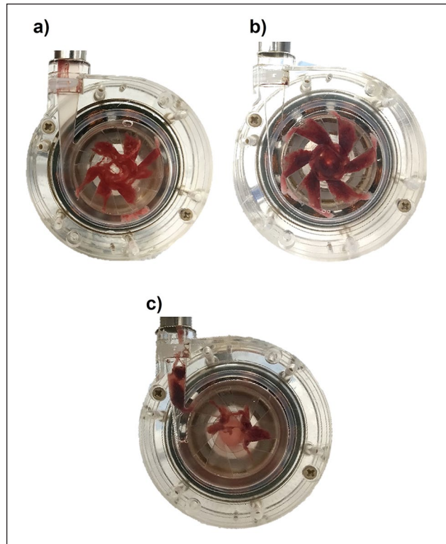
Figure 6. Observations of the pump after the thrombus detection tests. A thrombus was observed in the pump and no thrombus was observed in the RC for each of the three tests: (a) a 0.6 mL thrombus was observed after Test 1, (b) a 1.1 mL thrombus was observed after Test 2, and (c) a total of 1.0 mL of thrombus was observed after Test 3. A 0.2 mL thrombus was found near the centre of the pump as in Tests 1 and 2. The remaining 0.8 mL thrombus was found at the volute outlet of the pump.
