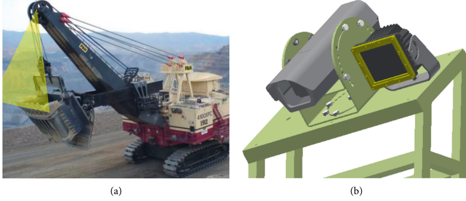
FIGURE 1: Illustration of our proposed solution on automatic electric shovel teeth detection.
