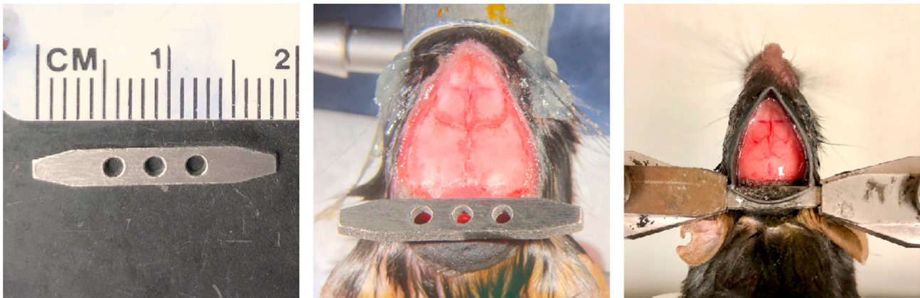
Figure 2. The custom-built stainless steel headbar (left) attached to the skull (middle) for head fixation on the stage (right) under the wide-field microscope
