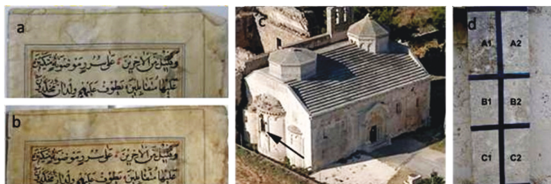
FIGURE 19: Conditions of old manuscript (a) before and (b) after coating with ZnO NPs, (c) building for the in situ experimentation of coating, and (d) the tested area results between coated and uncoated parts. Illustration was taken from Ref. [24].
