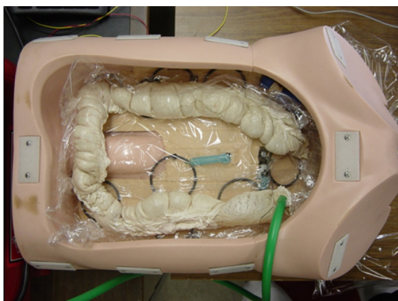
Figure 14 Colonoscopy training model with porcine colon. Air is inserted to open the lumen for more realistic intubation.
