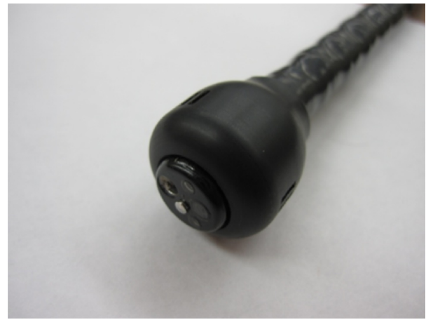
Figure 3 Sensory system of the colonoscopy add-on device.
