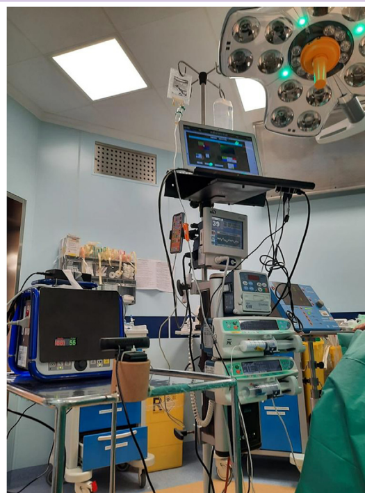
Fig 1. TI.VA prototype. The components of the first prototype system for managing the TI.VA algorithm are shown. The MacBook® screen shows the user interface constructed using a number spreadsheet (Apple Inc., Cupertino, CA, USA). The same stand holds the BIS™ monitor (Medtronic, Dublin, Ireland) and the Alaris® Gateway Workstation (Becton-Dickinson, Co., Franklin Lakes, NJ, USA), with two target-controlled infusion pumps dedicated to propofol and remifentanyl administration. Communication of the Alaris® workstation with the MacBook is enabled using an Ethernet port, while communication with the bispectral index system is achieved using an RS232 port. The CNAP® monitor (CNSystems Medizintechnik GmbH, Graz, Austria) is connected via a separate port. In this case, the implementation of a communication interface with numbers is more problematic. Thus, we ultimately decided on optical character recognition technology guaranteed by a camera mounted in front of the monitor. The monitor screen is masked to optimise the recognition process. Data (i.e. mean arterial pressure and heart rate) are shown in the window directly in front of the camera. TI.VA, total intravenous anaesthesia.
