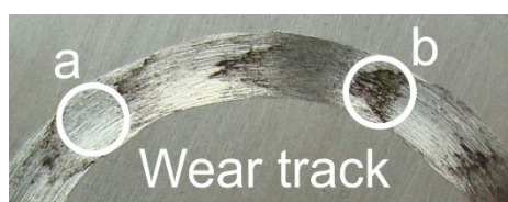
Figure 17. Corrugation wear on the friction surface (a—area with trace amounts of wear debris, b—area with densely packed wear debris).
