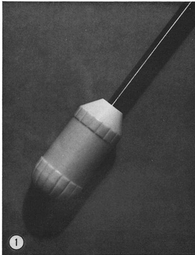
FIGURE 1 Specially constructed teflon homogenizing pestle. The middle two-thirds of the pestle was machined to provide an area of large clearance for use in the preparation of neurosecretosomes. The upper and lower segments center the pestle so that the central clearance dimension between teflon pestle and glass vessel wall is constant during homogenization. The grooves permit the pieces of tissue to pass into the central area of wide clearance where disruption occurs.
