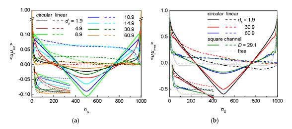
**Figure 10.** Orientation correlations for: a flexible chain (**a**); and a semiflexible chain (**b**) of circular and linear topology in an array of nanoposts of fixed passage width  $w_p = 2$  and various post diameters  $d_p$ . The insets zoom in the initial decay of the orientation correlations.
