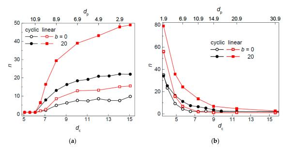
**Figure 3.** Occupation number of a flexible (b = 0) and semiflexible (b = 20) circular and linear chain in an array of posts of varying diameter  $d_p$  separated by  $S_p = 12$  (**a**) and with passage width  $w_p = 2$  (**b**) as a function of the size of the interstitial space.
