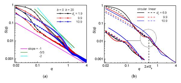
**Figure 8.** Structure factor for: a flexible and semiflexible circular chain (**a**); and for a flexible circular and linear chain (**b**) confined in an array of nanoposts of fixed post separation  $S_p = 12$  and various post diameters  $d_p$ . In (**a**), the solid lines represent the characteristic slopes that might be expected for a biaxially confined chain; and, in (**b**), the inset zooms in the region of humps with the vertical dashed line indicating its predicted onset.
