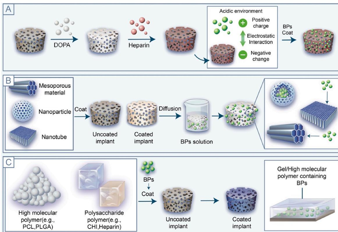
**Fig. 6.** BP-coating strategies. A) In an acidic environment, BPs that present a positive charge are coated on the negatively charged surface by electrostatic interaction. B) BPs can incorporate into porous materials, including mesoporous materials, nanotubes, and nanoparticles, to form drug coatings. C) High-molecular polymer and polysaccharide polymers encapsulate BPs to form composite coatings on the implant surface.
