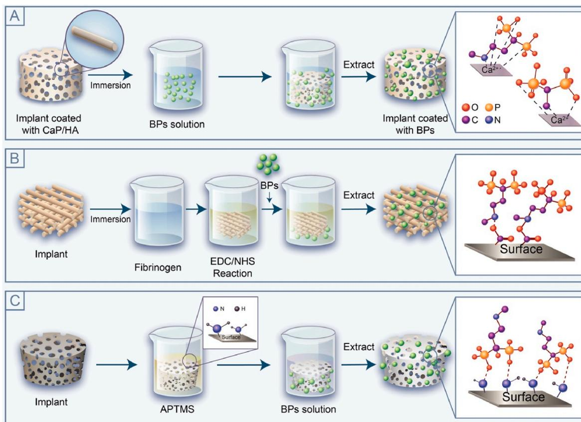
**Fig. 5.** BP-coating strategies. A) Binding materials containing calcium ions to the implant surface and immersing in BPs solution. B) EDC/NHS activated carboxylic group of fibrinogen surface binds to the amino group of N-BPs to form the BP coating. C) BPs coated on the implant by combining with the surface modified by APTMS.
