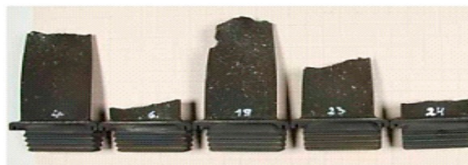
Figure 6. Cracked turbine blades.
