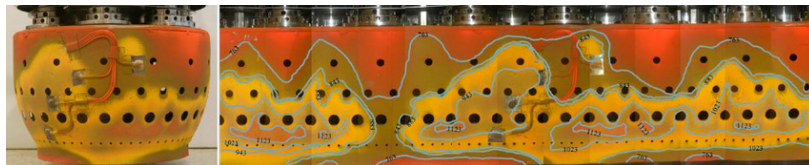
Figure 22. Thermal paint gradients of the combustor outer liner [199], with permission from Begell House, Inc.
