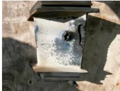
Figure 3. Overheated turbine vane.
