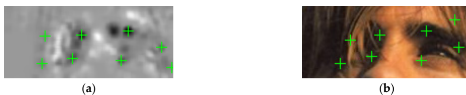
Figure 15. Failure cases of eye center localization. (a) Symmetry transform image and selected eye candidates; and (b) selected eye candidates (on the input image).
