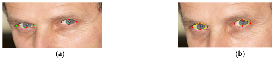
Figure 22. Difference between the annotated eye corners and the detected sclera landmarks. It can be noticed that even if the sclera is correctly segmented, there is a larger distance between the annotated eye corners and the sclera landmarks. (a) Annotated landmarks on LFPW database (in green) and detected sclera landmarks (in red); and (b) segmented sclera region.
