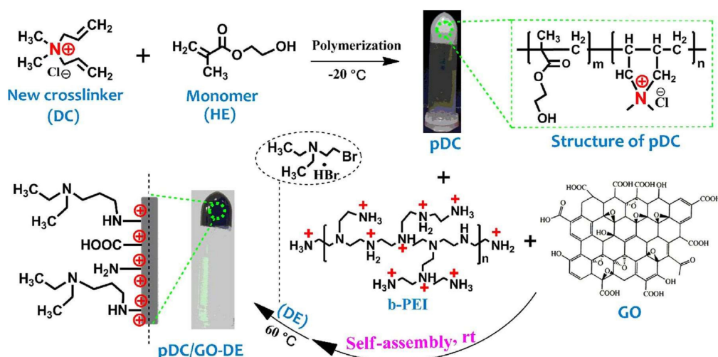
Figure 9. Scheme of composite cryogels preparation. Republished with permission from [61]. Copyright 2019 Elsevier.
