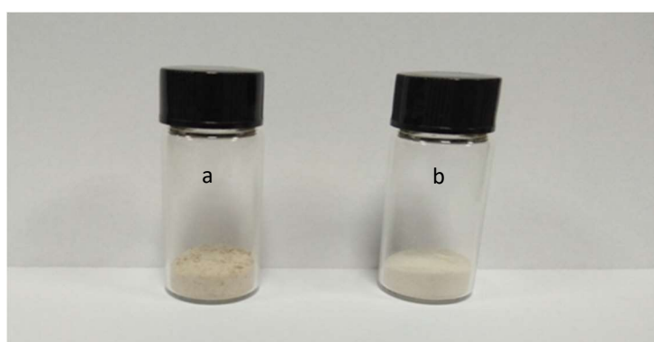
Figure 2. (a) Freeze-dried inulin sample and (b) spray-dried inulin sample.
